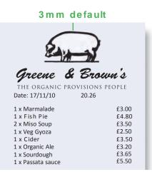
**80mm – 58mm Auto Reduction without changing original POS Software** The TSP100 ECO can automatically reduce receipts from an 80mm wide format to 58mm without changing the customer's original software set-up. Simply tick the required paper reduction in the ECO *futurePRNT* software and you can choose whether to reduce the receipt vertically or horizontally, or both to 72.5% horizontally and 50% vertically.
